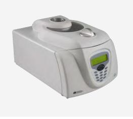
The Air Trace<sup>®</sup> Environmental Air Sampler continuously measures the viable microorganism counts within the test chamber and mechanical system
