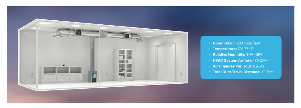
Test conditions represented an active mechanical system and indoor environment through a "Hot Start" scenario where the PuriFi product and HVAC fan system were activated 15 minutes before introducing the pathogen into the environment.
