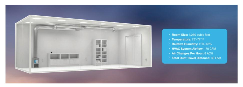
Test conditions represented an active mechanical system and indoor environment through a "Hot Start" scenario where the PuriFi product and HVAC fan system were activated 15 minutes before introducing the pathogen into the environment.
